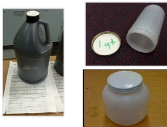
Figure 5 - Emulsified Asphalt Sample Container Options
