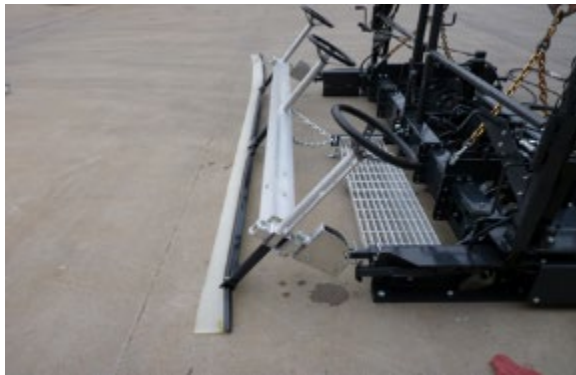
Figure 29 - Secondary Strike-Off on Variable Width Spreader Box (Spreader Box width is adjustable while applying mixture)
